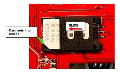
6. Slide the top frame to the left to lock the frame to the bottom.
