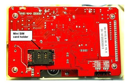
2. Slide the top of the card holder to the right. A gap will appear between the top and bottom of the cardholder.
