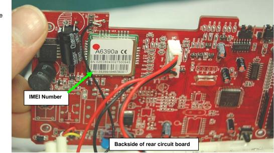
4. Record the IMEI number and carefully re-assemble the circuit boards.
