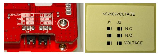
NOTE: The "VOLTAGE" jumper position is not used in conjunction with the E-xD.
