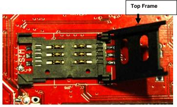
4. Insert the Mini SIM card into the slot on the top frame. The contacts should be facing you and the cut-off corner of the card should be towards the right. Insert the card all the way in until it stops.
