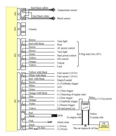
\*Orange with black wire of JP1: Engine status detection, it is used to detect the engine started or not after automatically start command, this wire connects to the power wire
