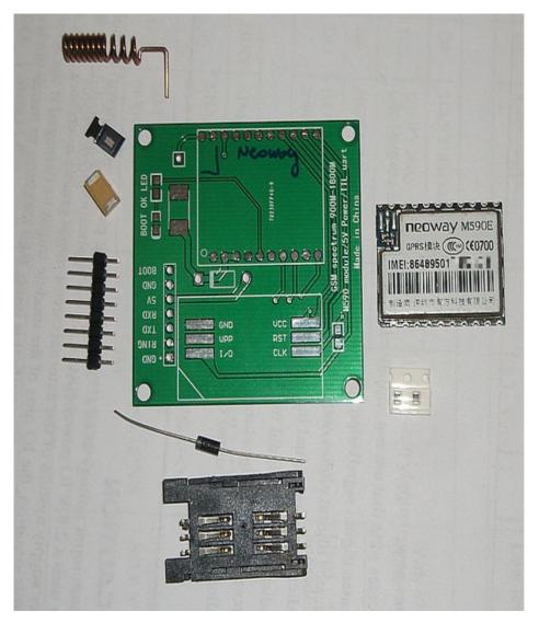
This instructable is about an extremely cheap GSM/GPRS module which comes as a do it yourself kit. We are going to assemble the parts and do some basic operations through software terminal. Finally we send out SMS messages.
