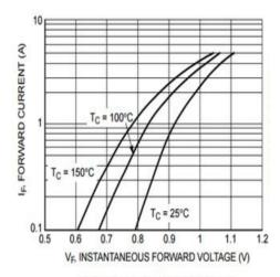
Figure 1. Typical Forward Voltage
