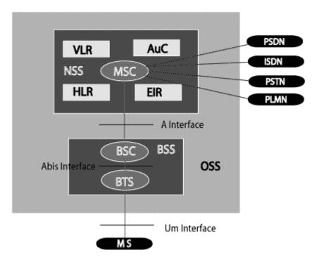
The additional components of the GSM architecture comprise of databases and messaging systems' functions:
