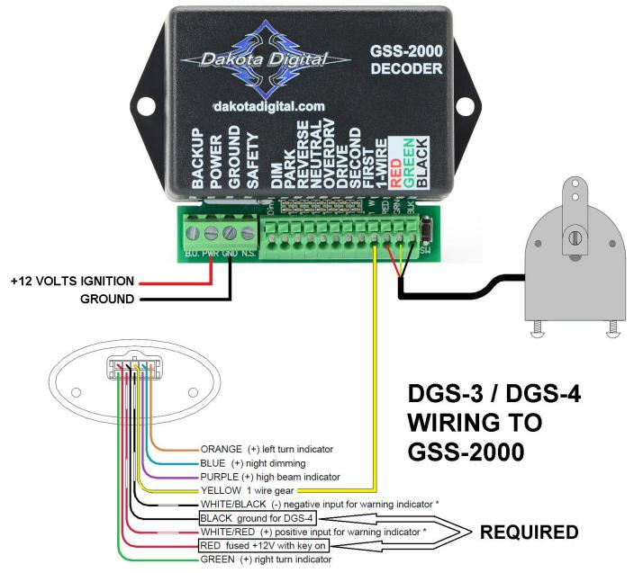
\*NOTE: Both warning indicator inputs must be used.
