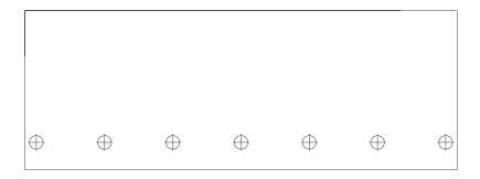
The universal mounting plate requires mounting holes be drilled to line up with the pan bolts on the transmission. This can be used with transmissions for which a specific mounting plate is not provided.
