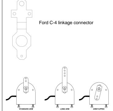
The arm on the gear shift sender will need to be flipped around so that it rotates on the bottom half. Make sure that the slot in the shaft is in line with the sender arm as shown in the diagram.
