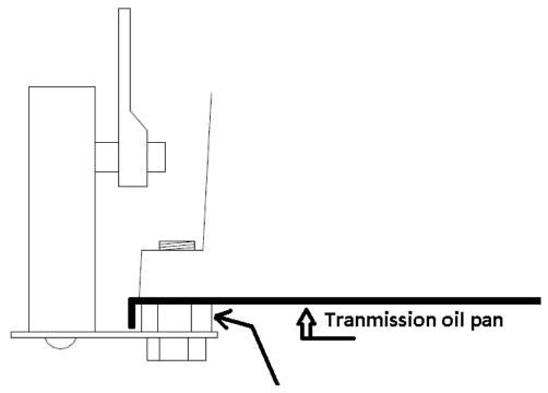
Use the 5/16" x 1" bolts, and 7/16" nuts (acts as a 3/8" spacer) as shown, to mount the plate to the transmission pan
