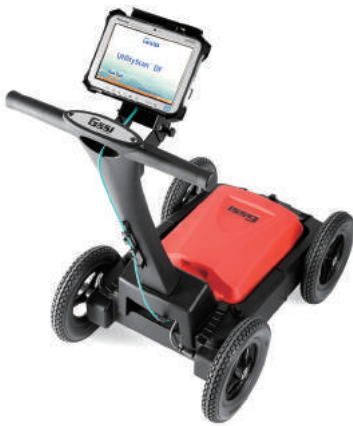
Compact Survey Cart
