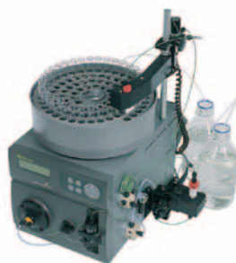
Fig 6. Purification of GST fusion proteins using a GSTrap FF column and ÄKTAprime.
