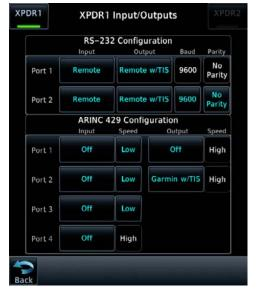
Figure 5-33. Remote XPDR Inputs/Outputs Page
