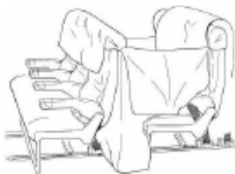
Fig1: example of installed CSB ready to be loaded
