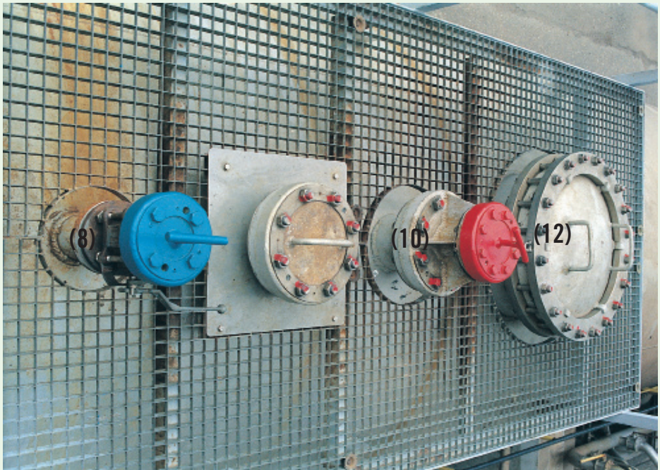
Fig. 2 Tank wagon fittings at the top (red rising pipe, blue pressure nozzle). In this example the rising pipe is without a shut-off valve
