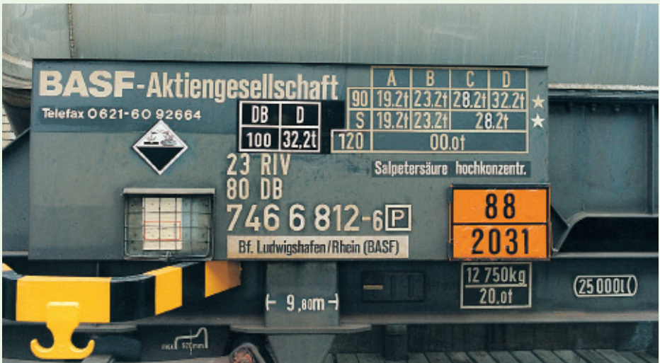
Fig 7 Dangerous goods marking of a tank wagon containing nitric acid Class 8, 2a) 1 RID (nitric acid other than non-red fuming and greater than 70%)
