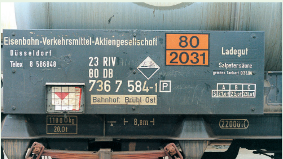
Fig 6 Dangerous goods marking and labelling of a tank wagon containing nitric acid Class 8, 2b) RID (nitric acid other than non-red fuming and less than 70%)
