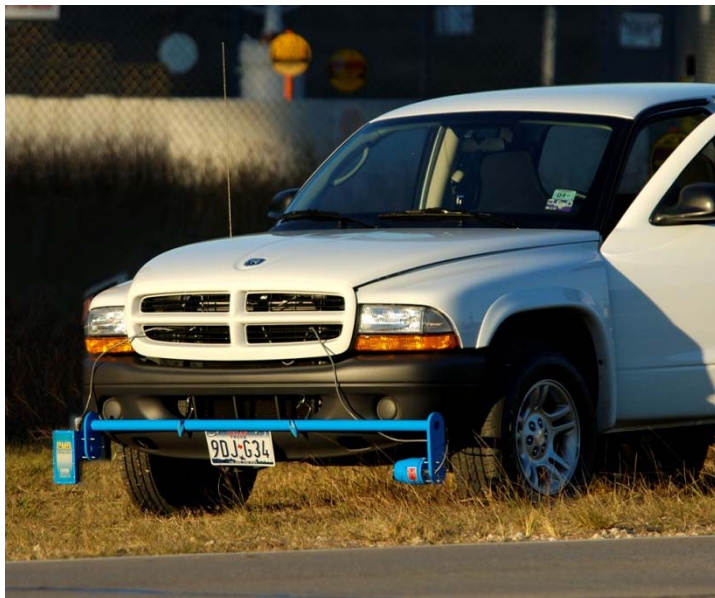
Figure IV-5: Optical Mobile Methane Detector
