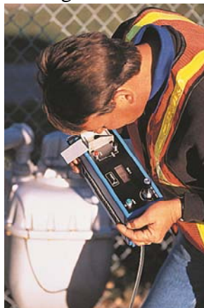
Figure IV-10: Conducting a Sniff Test Using an Odor Testing Instrument.
