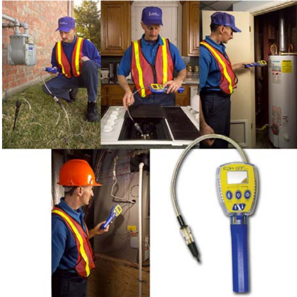
Figure IV-3: Combustible Gas Indicators. Photos courtesy of Heath Consultants, Inc.
