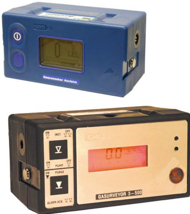
Figure IV-3: Combustible Gas Indicators. Photos courtesy of Heath Consultants, Inc.
