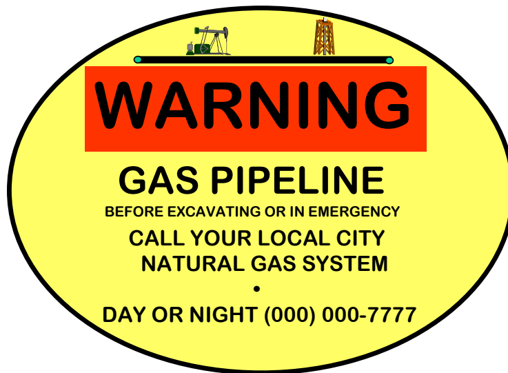
Figure VIII-2: Pipeline marker that meets the federal requirements
