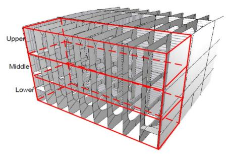
FIGURE 3 Areas under Consideration for a Wing Ballast Tanks of a Single Hull Tanker
