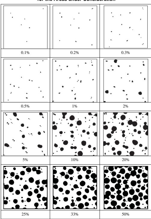
FIGURE 1 Diagrams of Scattered Coating Breakdown for the Areas under Consideration
