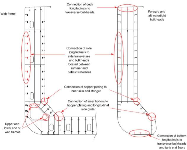
FIGURE 8 Typical Critical Areas in a Double Hull Tanker
