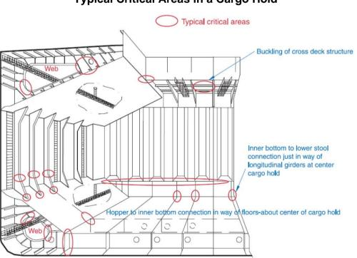
**FIGURE 11 Typical Critical Areas in a Cargo Hold**
