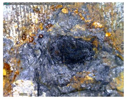
FIGURE 4 Typical Pitting Corrosion
