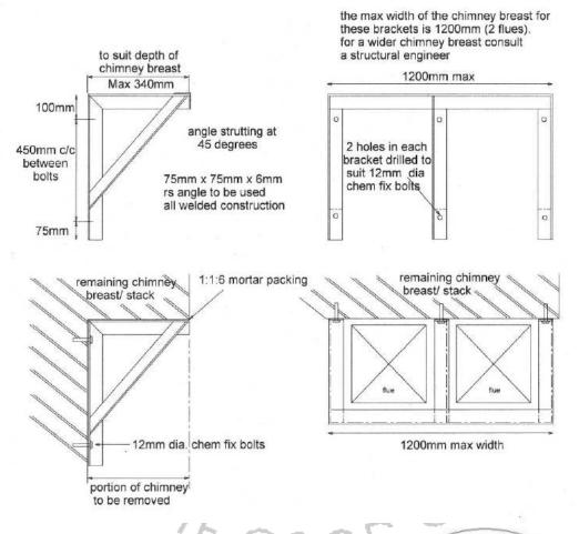
It is recommended that the top member of the gallows bracket is extended by 100mm in order that it can be built into the existing brickwork.
