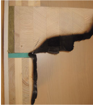
Figure 27: Fire test with elastomer vibration absorber in wall to floor junction, (Teibinger 2011, Merk 2014)
