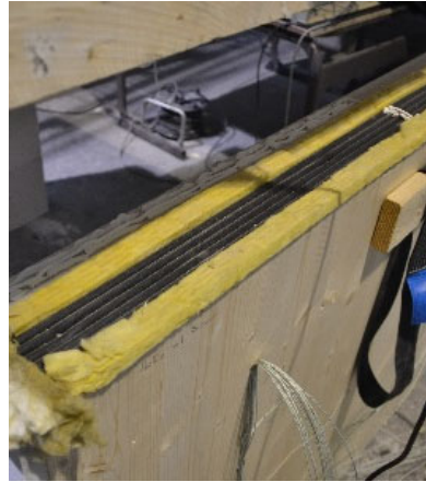
Figure 27: Fire test with elastomer vibration absorber in wall to floor junction, (Teibinger 2011, Merk 2014)
