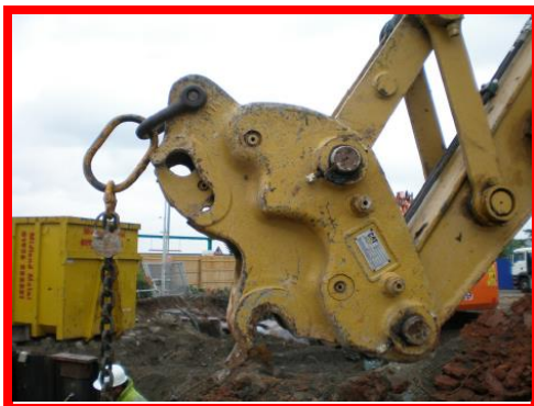
Figure 14. – Hitch tilted backwards with master link subject to bending
