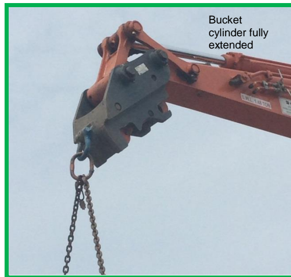
Figure 13. – Chain and master link can hang freely without obstruction
