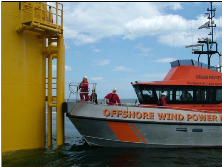
Figure 6 – Personnel transfer from a CTV to an offshore wind turbine boat landing (photo: Workships Contractors)
