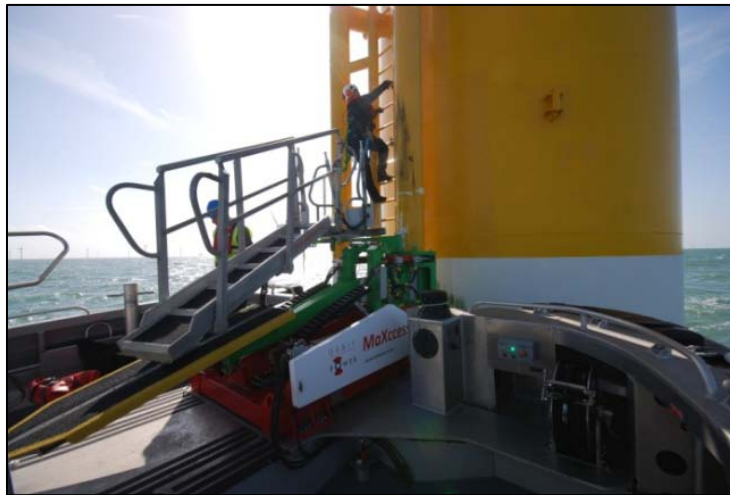
Figure 8 – Personnel transfer from a CTV using a transfer access system (photo: Osbit Power Ltd)
