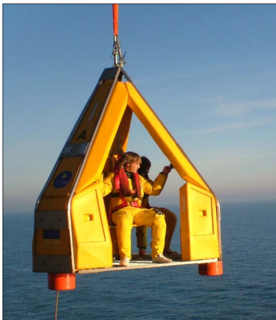
Figure 2 – Personnel transfer using a transfer capsule (photo: Reflex Marine)
