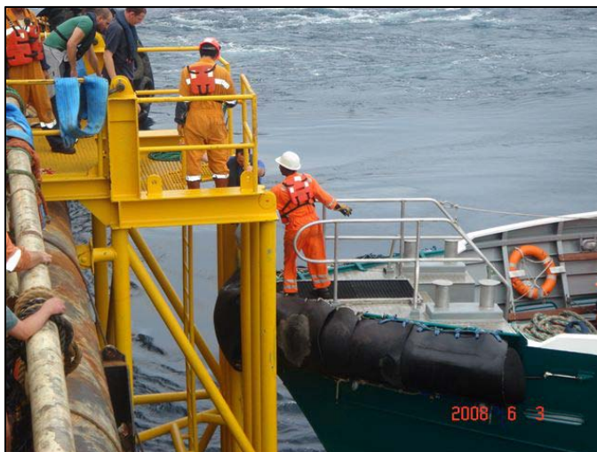
Figure 5 – Personnel transfer from a crew boat to a larger vessel using a 'surfer' (photo: Saipem)
