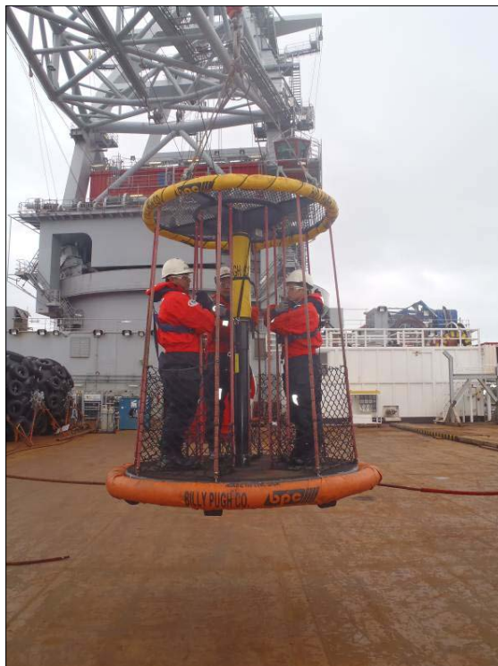
Figure 1 – Personnel transfer using a rigid basket (photo: Seaway Heavy Lifting)
