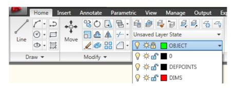
AutoCAD is a drawing program but it uses a virtual space. Therefore drawings can (and should) be drawn at full 1:1 scale.
