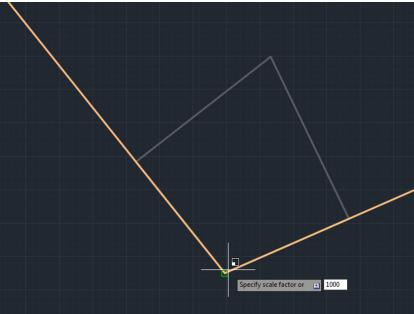
Before you can take the drawing into illustrator or printing you have to convert the drawing into millimetres. Since you probably drew your drawing in metres you simply have to scale the drawing up 1000 times (since 1 metre is 1000 millimetres)
