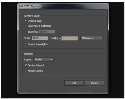
Save your AutoCAD drawing as the native dwg format but make sure it is in the older dwg2000 version (AutoCAD 2000/LT2000 Drawing). This is because the newer versions of dwg contain 3D information which causes problems when transferring to Illustrator.
