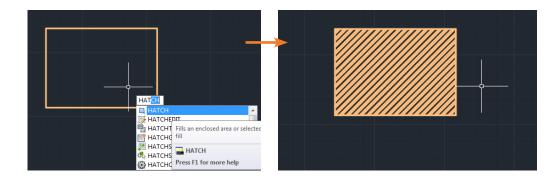
**(HATCH or H)** - By executing this command and clicking the centre of a shape, a hatched texture is created. Useful for distinguishing different surfaces/textures
