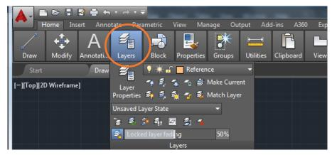
A drawing can (and should) be organised into layers in order to make it easier to manage. It allows the option to turn layers on and off as well as lock layers to prevent accidental selection of editing.
