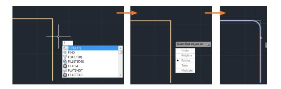
(FILLET or F) - This tool can be used for rounding/ curving existing corners with a specific radius. Type 'F' then press the 'down arrow' button. Select 'Radius' and type the radius measurement you want. Press Enter. Then click the lines where you want the corner to be rounded.
