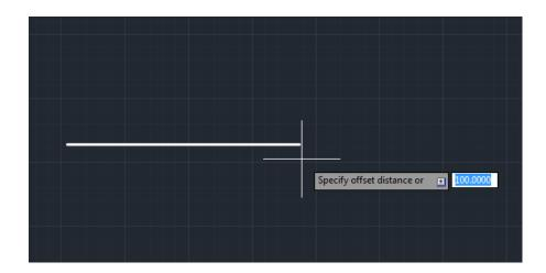
Offset is a very useful tool for creating copies of objects at specific distances apart (e.g. for wall thickness). It can also be used to create temporary guidelines for creating other objects.
