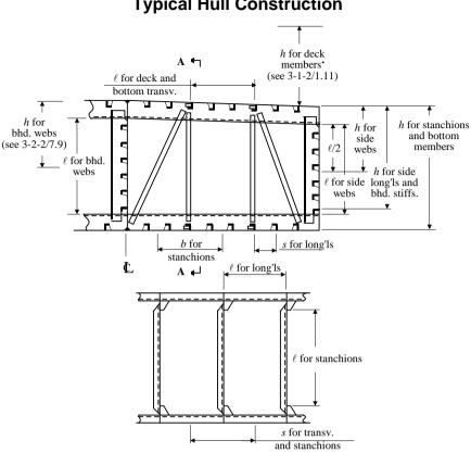
FIGURE 1 Typical Hull Construction
