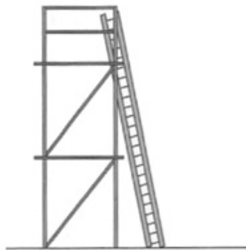
Extension ladder set against a scaffold
