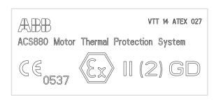
Parentheses indicate that a safety device can be used to protect products with equipment categories 2 and 3, but the safety device itself and the drive where it is integrated must be installed in a safe area.
