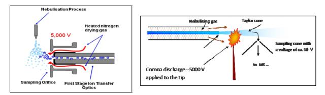
Figure 2.3: Schematic of ESI source
