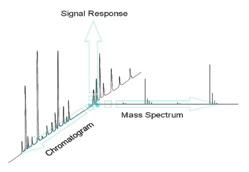
*Figure 1.1: The power of the LC-MS technique to separate and identify each component of a complex mixture*
