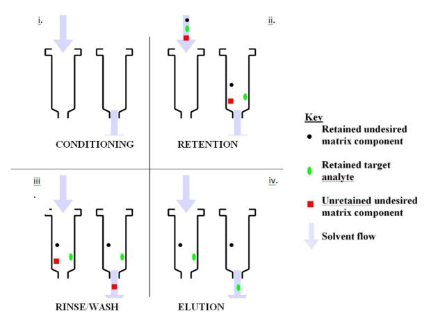
Figure 4.3: Generic experimental workflow for an SPE extraction showing the retention and separation of the target analyte from other components in the sample.
