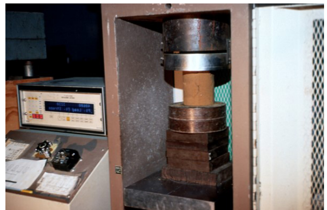
Figure 2.4. Unconfined compressive strength test being performed on an FDR with cement specimen
