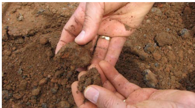
Figure 7.4. Hand-squeeze moisture test
