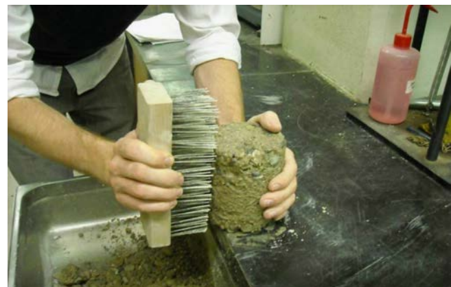
Figure 5.10. Brushing during freeze-thaw durability testing
