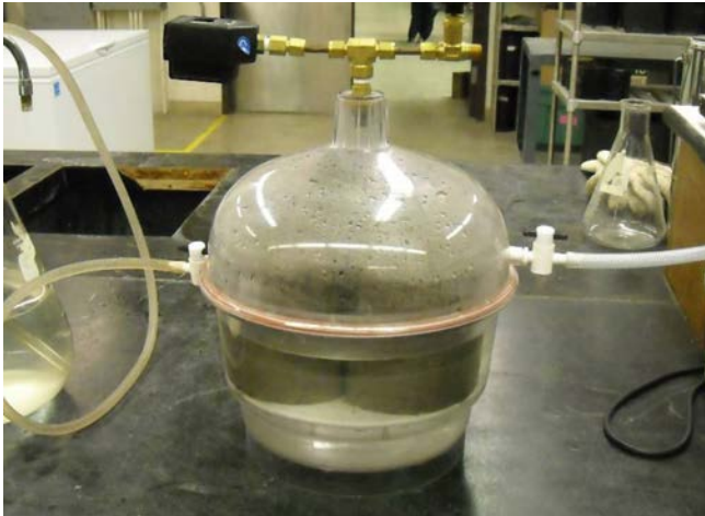
Figure 5.11. Vacuum saturation test
