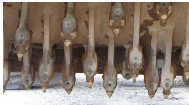
Figure 6.3. Roadway reclaimer cutting drum
