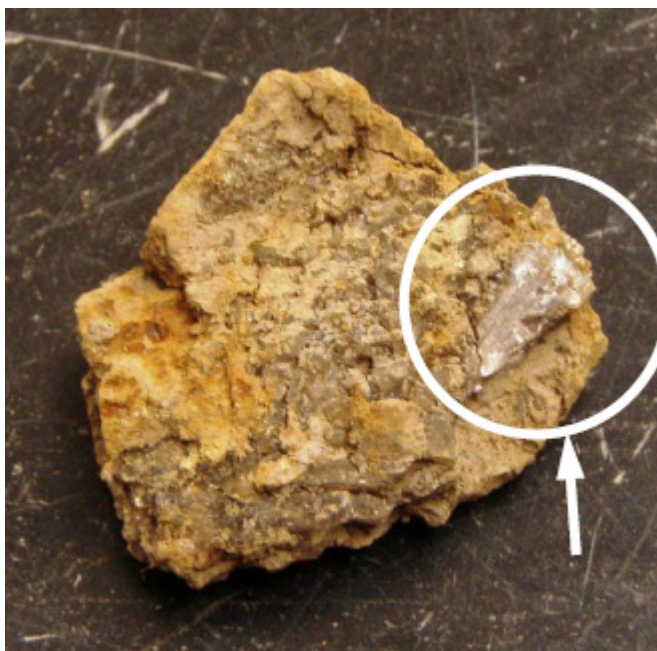
Figure 5.7. Gypsum crystal in clay
