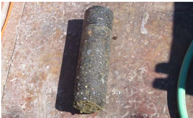
Figure 2.1. Core of FDR with cement base and HMA surface course
