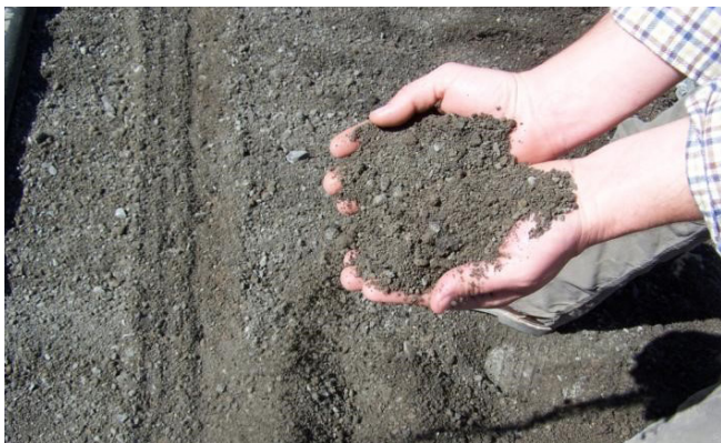
Figure 6.14. Pulverized FDR mixture
