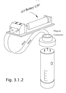
For gas sensors with TG no.'s: 170/270/880/1560 and 1750 the "BIAS voltage control" is activated through a 1.5 Volts battery device, see fig. 3.1.2.
