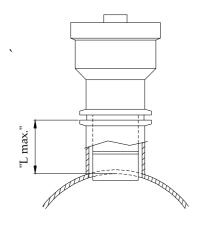
To ensure that the sensor is sufficiently in contact with the flow of air/gas, the flange should have maximum depth "L  $\max$ " as illustrated (see fig. 3.3.1)
