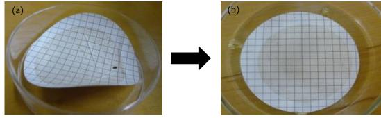
Figure 2: Glue procedure: (a) Curved filter; (b) Glued filter.
