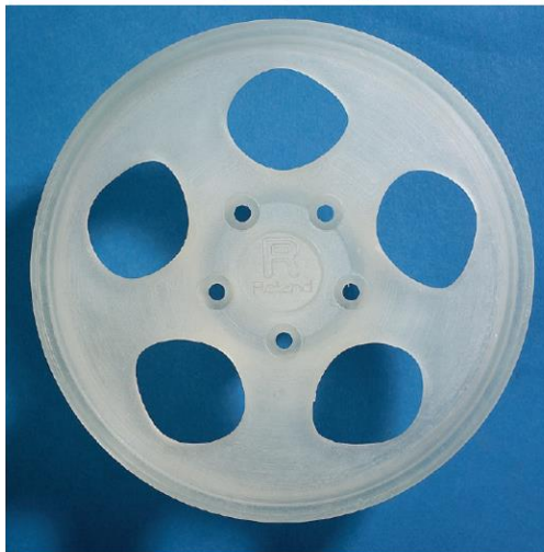
Acrylic wheel milled using Subtractive Rapid Prototyping (SRP).
