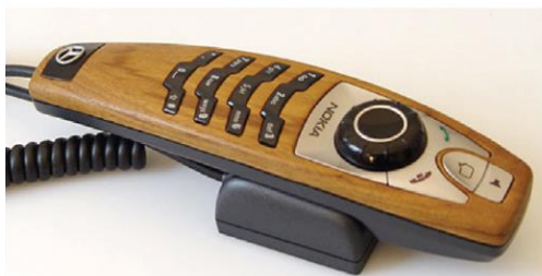
Finished phone prototype with wood, ABS and aluminum parts milled by the MDX-540.
