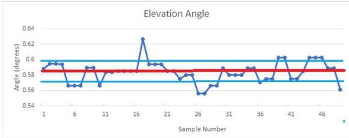
Figure 117. High resolution elevation data showing digitization
