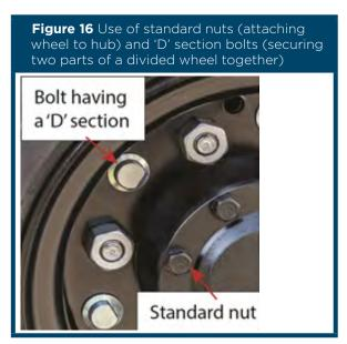
**Hub** means the assembly on the vehicle to which the wheel is fitted.
