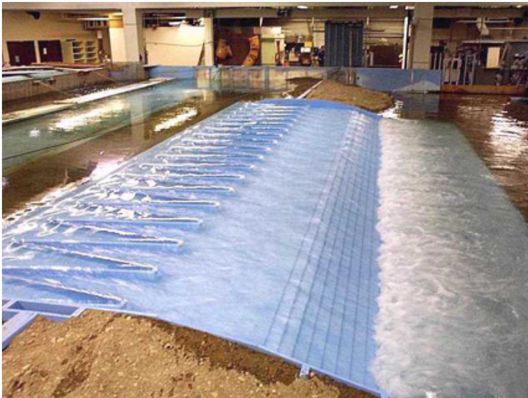
Figure 8: Labyrinth weir leading onto a stepped chute model, Lake Turner Dam, Texas. Photo from Utah State University Water lab website.
