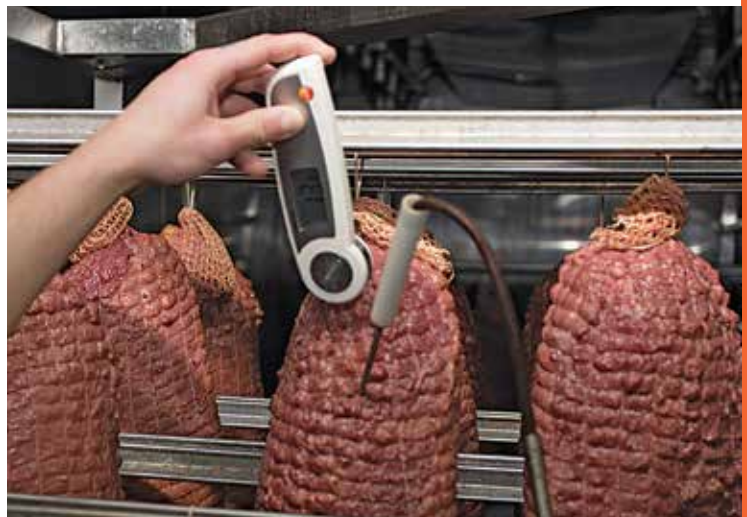
Figure 4.2 Checking the temperature at the slowest heating point using a hand held temperature probe
