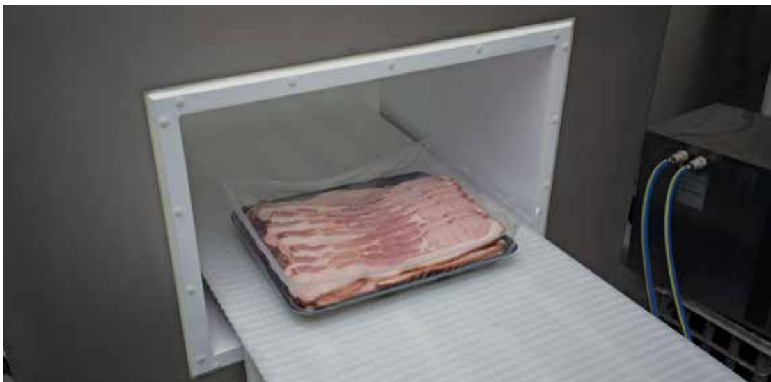
Figure 6.3 A pack of sliced bacon being put through a metal detector
