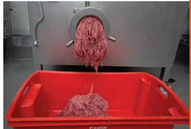
Figure 6.2 Grinder producing minced meat
