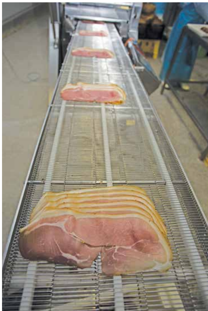
Figure 6.7 Conveyer belts are difficult to clean
