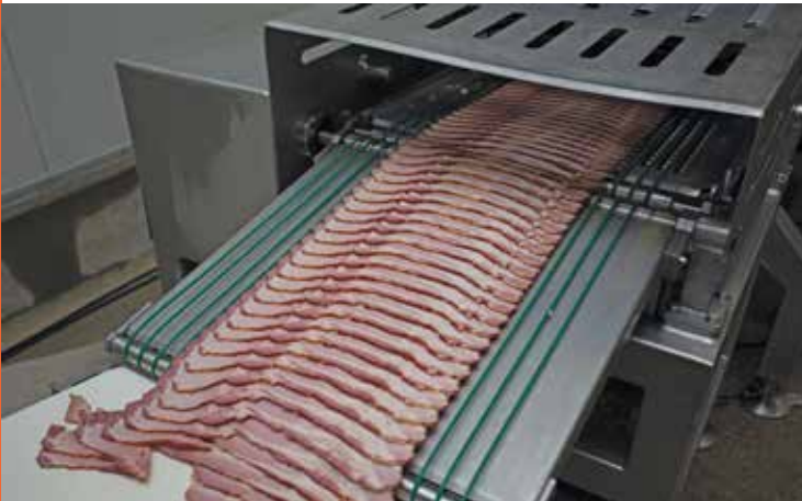
Figure 3.5 A slicing machine producing sliced bacon
