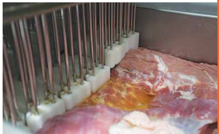
Figure 3.4 Injectors pumping brine into pork during bacon production
