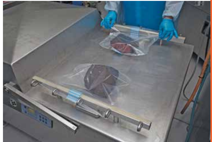
Figure 6.6 Manual vacuum sealer
