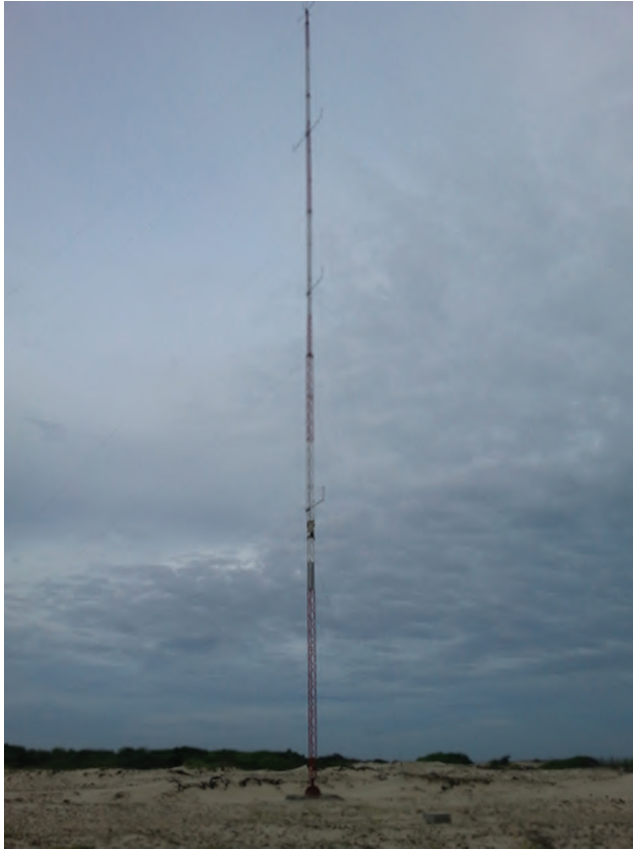
An 80-meter met-mast in Mannar, Sri Lanka. The measurement project is funded by the Asian Development Bank.
