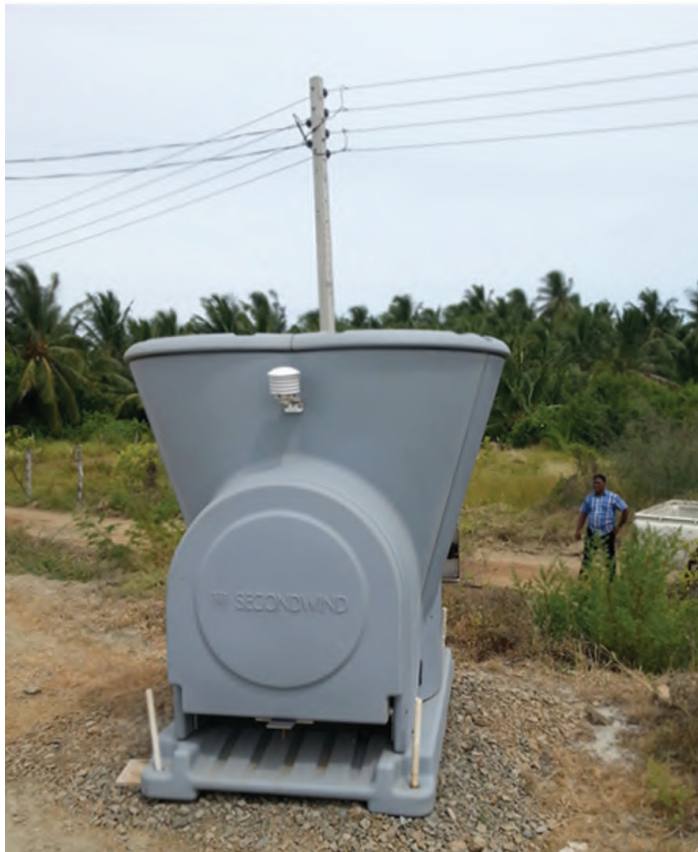
Sonic Detection and Ranging (SODAR) at the PowerGen wind farm in Sri Lanka.
