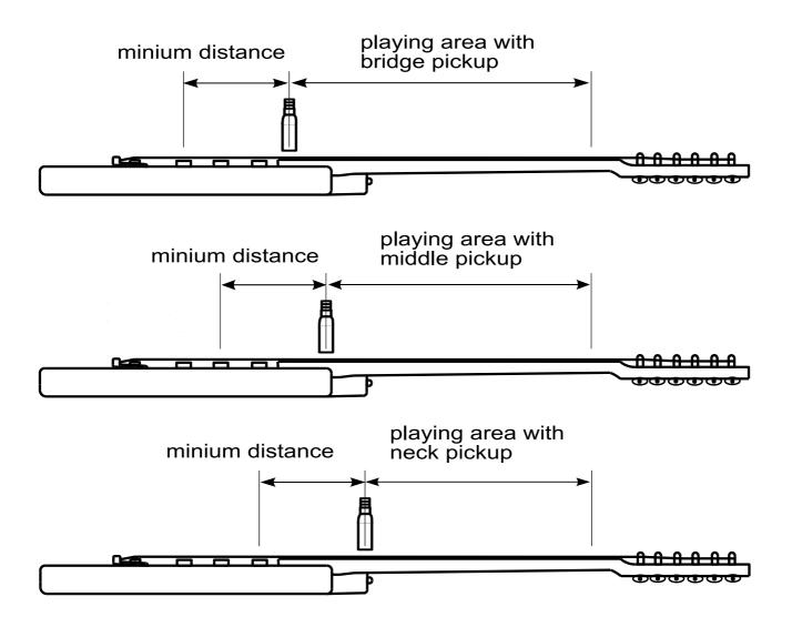
The sensitivity not only depends on the Resonator power but also on the pickup. In generell humbucker show less sensitive than single coils. With some practice you play closer by the strings which enables you to reduce the Resonator power. Then, you can also play with the neck pickup (or middle pickup). You should absolutely work it out, because these feedbacks are sounding very rich and amazing !
