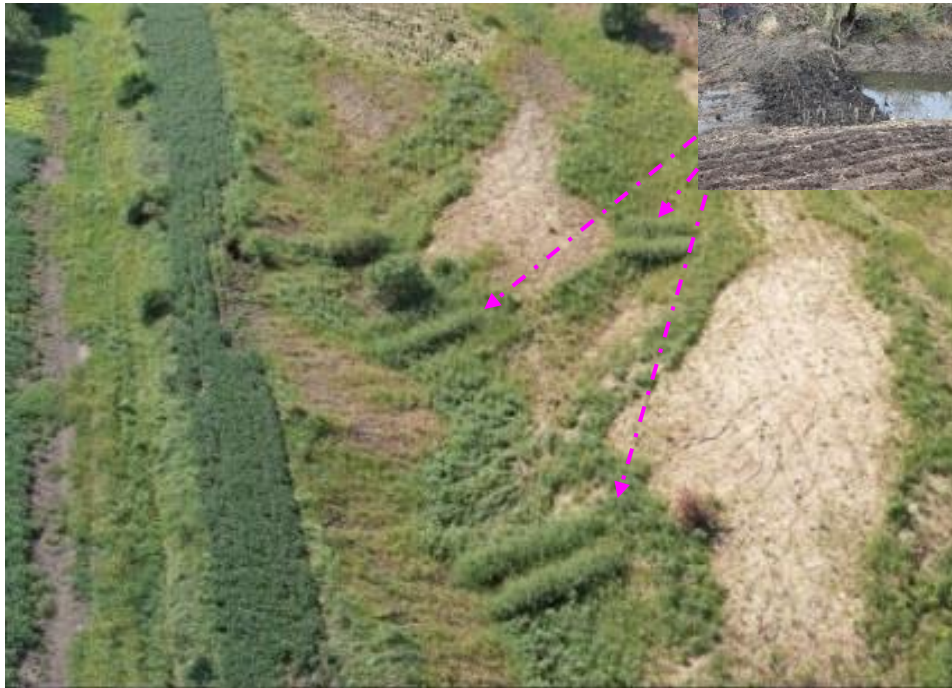
Figure 11. Typical wicker check dams (upper right corner, check dam establishment) (photo taken by Dr. X.Y. Zhang in July 2018, Kaiyuan City, Liaoning Province).
