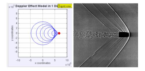
Unlike the sonic boom from an aircraft, this *crack* noise is audible only for a distance of some 30-50 meters (about 100-165 feet) away from the path of the bullet, and only for so long as that bullet travels supersonic (faster than the speed of sound). Inevitably, the bullet slows down due to air resistance (or due to impact), at which time the crack is no longer audible.
