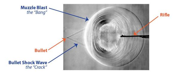
The *muzzle blast* is the noise we commonly associate with gunfire. It is the Hollywood gunfight sound effect that goes *bang*. Unless a suppressor is used, all guns produce a
