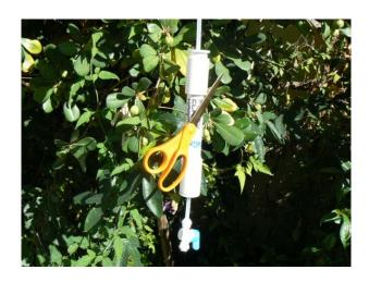
This photo shows that the magnets in the processor are strong enough to hold up a pair of scissors. The ¼ inch tubing is small enough to focus a very strong magnetic field from the ten rare earth magnets on the water flowing through the tube.
