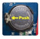
Step5: Get a new battery with the side of "CR2032" facing up, and install it to the mainboard.
