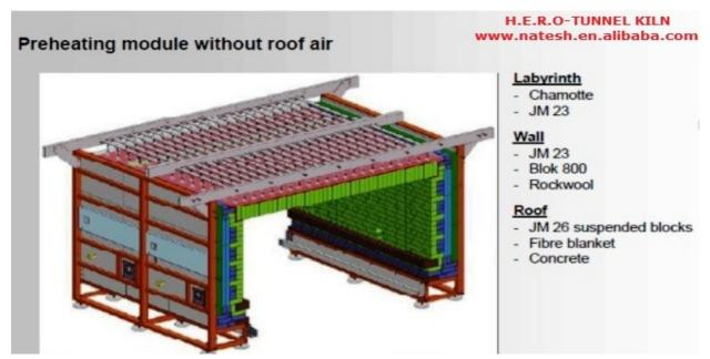
8. At the preheating zone, there are ducts with dampers for moisture discharge and can adjust the temp curve effectively in preheating.
