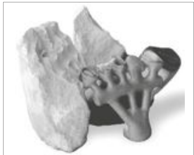
Fig. 18-39 Casting upon devesting Note the smooth, matte surface of the casting and its reproduction in the investment. Picture courtesy of PxDental Corp.
