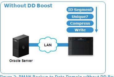
Figure 2: RMAN Backup to Data Domain without DD Boost
