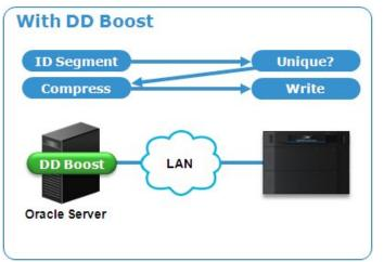
Figure 3: RMAN Backup to Data Domain with DD Boost
