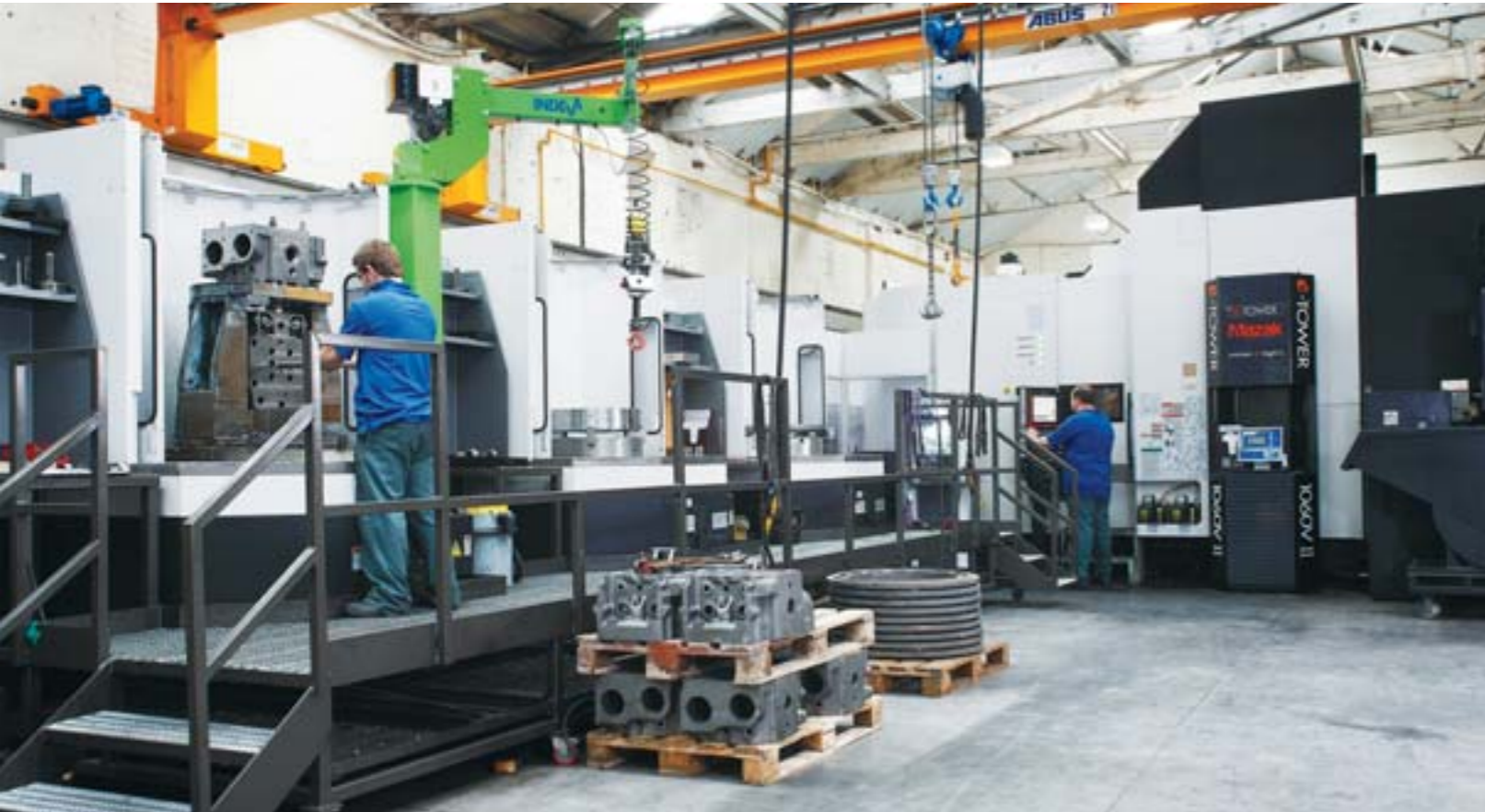
John Hyde Engineering's FLEXIBLE MANUFACTURING SYSTEM (FMS) in use with an INTEGREX e-1060V II.
