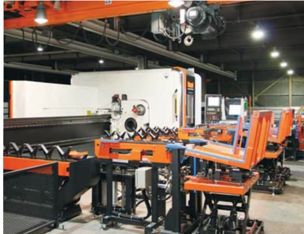
Material supply/loading system developed by Korenaga Shoukai for 3D FABRI GEAR 220 II
