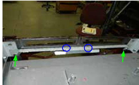
Lift light assy bracket off bolts to install bulb Remove two screws in locations shown
