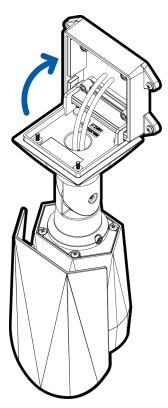
b. Use the camera mounting screws to fasten the camera to the bracket.
