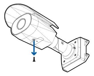
2. Remove the cover from the configuration panel.
