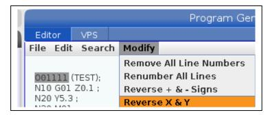
The Modify tab gives the option of putting in block numbers in a program. Also +/-signs and the X and Y may be reversed.
