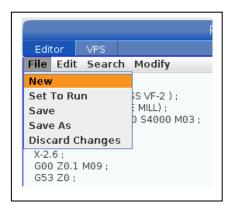
In the File drop down a **New** program may be created by high lighting New and pressing enter. Any editing changes can be saved by lighting **Save** and pressing enter. If a program needs to be duplicated the **Save As** function can be used. The Discard Changes function will undo all the current edits.
