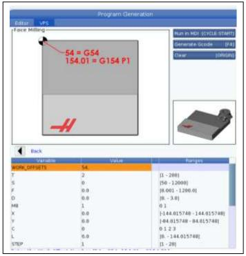
Key in the appropriate information such as work offset, tool, feed and speed, hitting enter. Pictures will pop up to give you information on what is needed to create the code. When you get to variable C it gives the different tool paths that may be created. When you pick the tool path desired then the X and Y values are the distances from your part zero to the corner one is starting from. For 0 the starting corner is the upper left hand corner.
