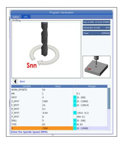
Below the depth, peck length, feed and thru the spindle coolant (M88) are indicated. M gives the different hole placement options that may be used. In option 1 the X and Y locations of all the holes may be given. Option 2 bolt circle with holes equally spaced may be
