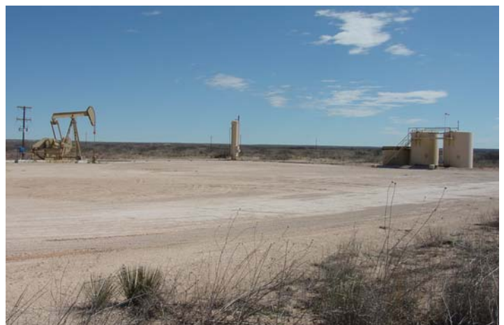
Figure 50. Typical oil well pad and associated structures with an overall footprint of the pad approximately 1-2 acres in size (Photo courtesy of NMDGF).
