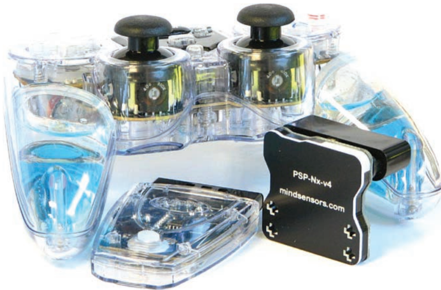
FIGURE 3.10 Mindsensors' PS2 adapter lets you control your model with a game controller.
