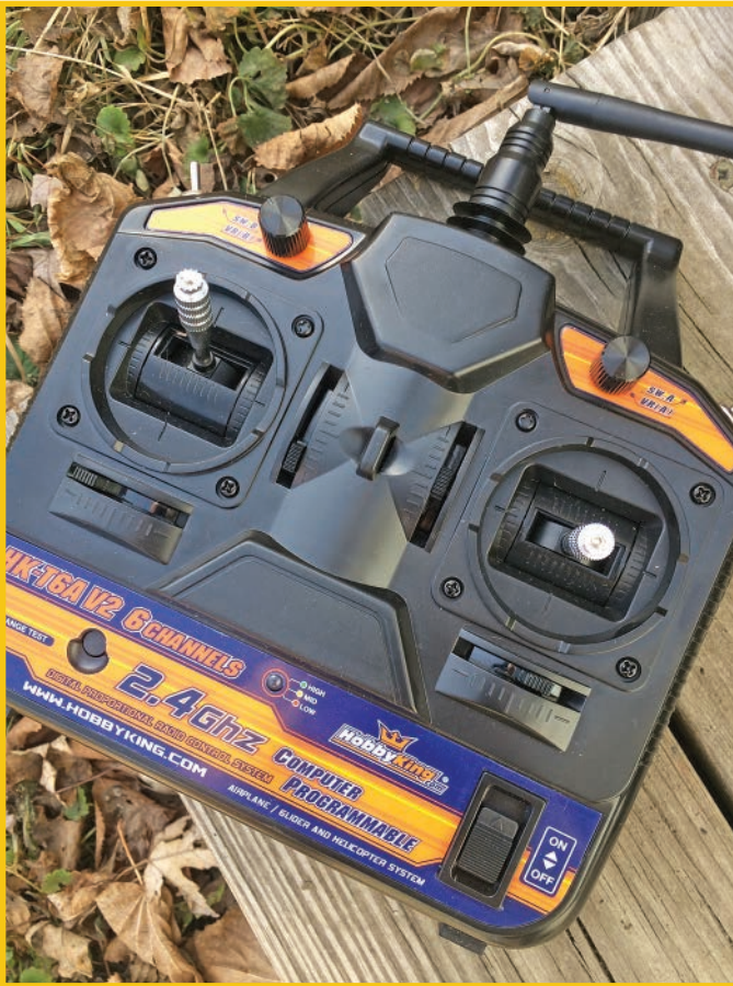
FIGURE 3.9 An RC transmitter and receiver can control Mindstorms models.
