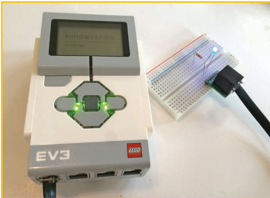
FIGURE 3.4 To access the inner wires individually, use a breakout board.
