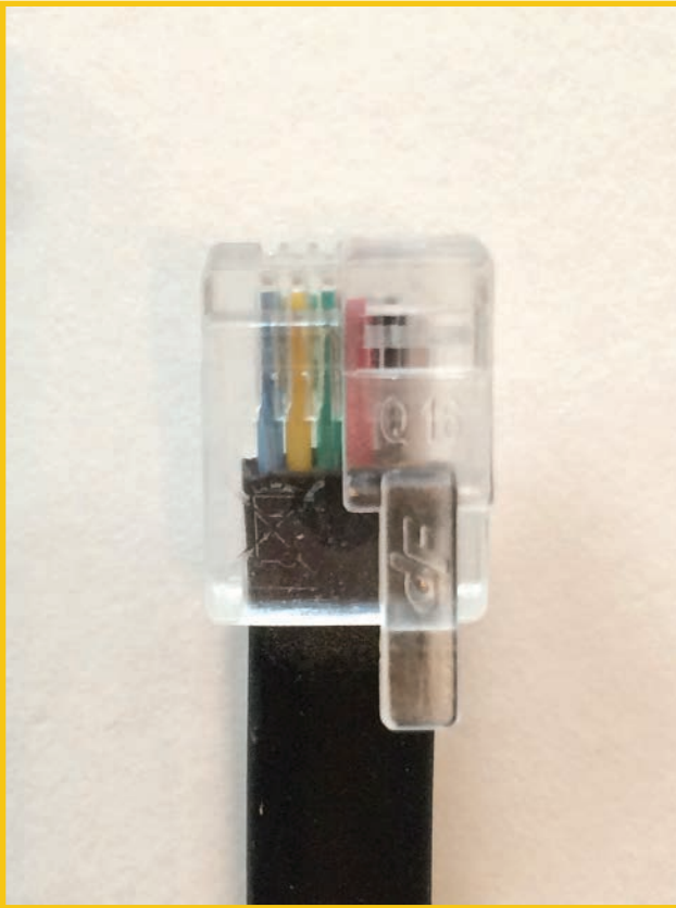
FIGURE 3.1 Mindstorms cables' off-center tabs are all that differentiate them from RJ12s.
