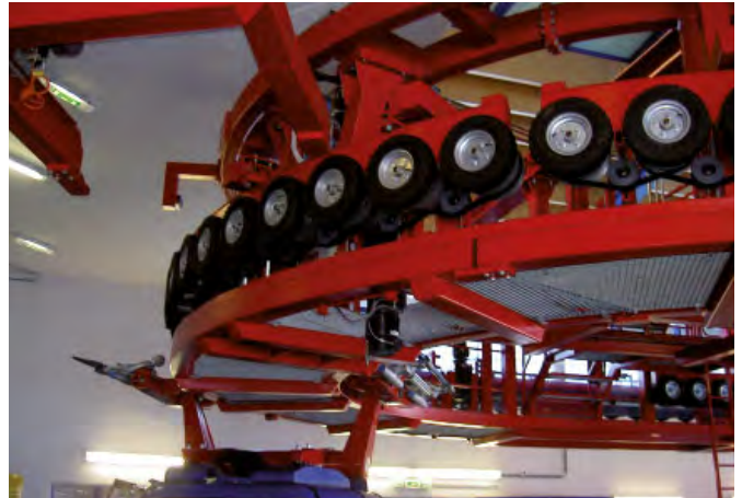
Fixing of the drive unit for a ski lift
