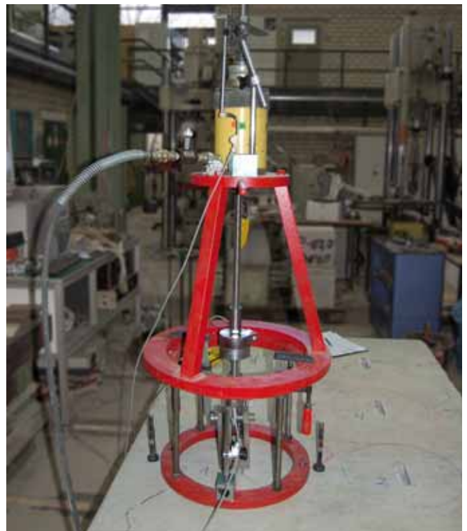
Test setup; pull-out test
