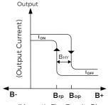
(Magnetic Flux Density B) Inverted South Pole Active
