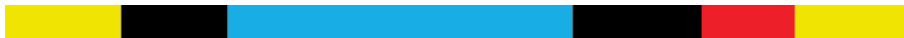
Figure 6 Content of target-enriched amplicons. Each amplicon contains one target insert (blue) surrounded by the Illumina paired-end sequencing elements (black), the sample index (red) and the library bridge PCR primers (yellow).
