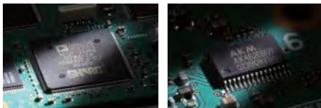
<DSP unit> ADSP-21369 Internal clock speed: 333MHz 32-bit floating point DSP Max. performance: 2000MFLOPS
