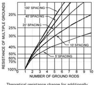
Theoretical resistance change for additionally spaced ground rods.
